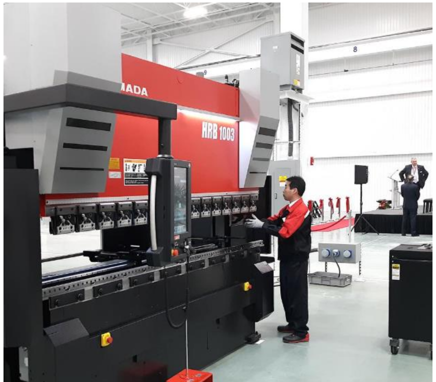
A worker demonstrates the operation of a press brake machine, which is used for precision metal bending, during Amada's ceremonial opening.
